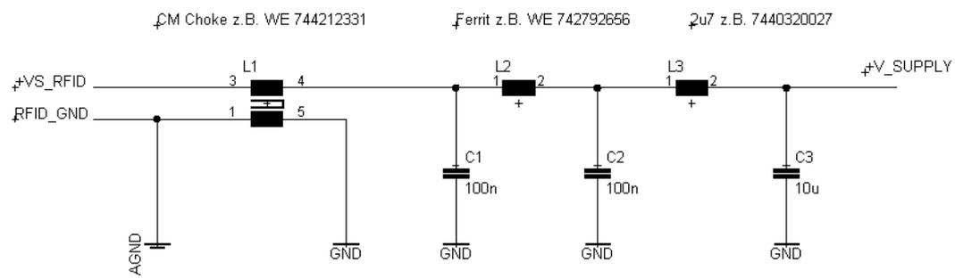
Fig. 4: Schematic for additional EMC filtering
