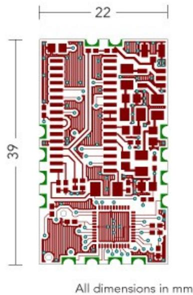
Fig. 3: Dimensions of Dwarf14 (in mm)
