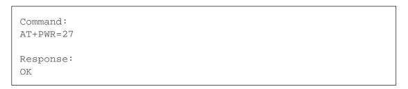
Besides setting a single output power for all antenna ports, you can also define separate output powers for each antenna by just adding more power parameters until you reach the number of antennas of your current setup. This includeds any connected multiplexer ports. Devices with only one antenna port and no outputs (DeskID UHF and QRG2) do not support multiple values for power.
